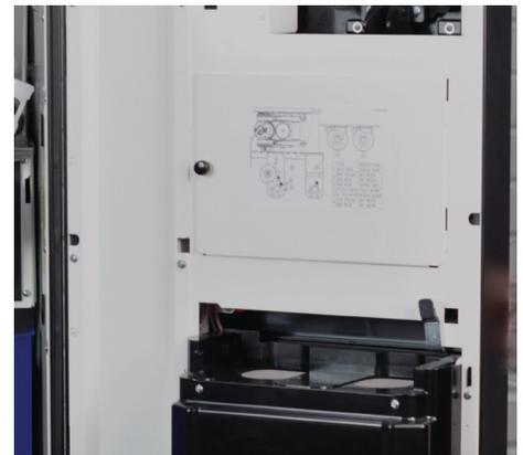
4.7 Return grounds tray container to machine. Reattach drip tray assembly to bottom and close door.
