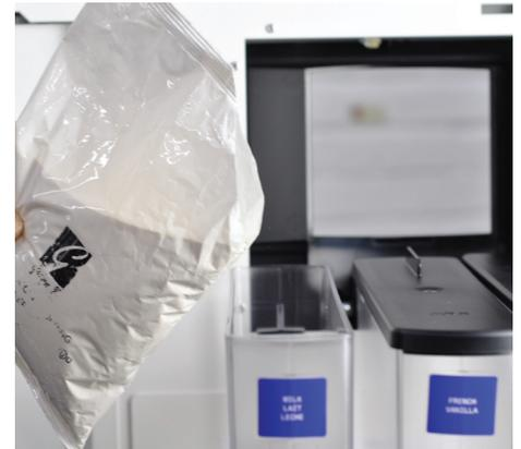
2.4 Wipe interior shelf with a clean dry cloth. Then, return filled canister(s) to machine, ensuring that tab on top of each canister fits in its corresponding guide slot as shown. Push each nozzle down.
