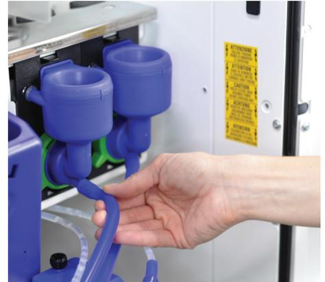
4.6 Remove waste bucket. Then, wipe waste bucket tray with dry cloth and then clean lower part of machine and inside of door.
