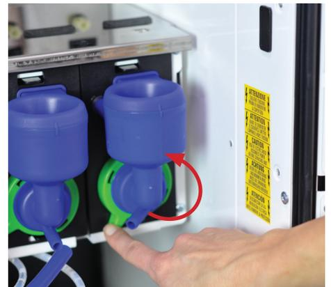
4.3 Firmly pull mixing bowl forward to remove from machine. Then, remove powder trap.
