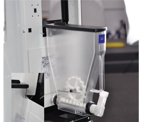
4.2 Disconnect blue tubes from mixing bowls. Then, for each mixing bowl, turn green ring counterclockwise about 1/8 turn.
