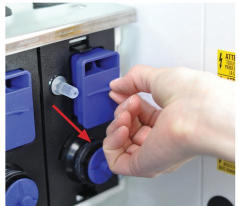
4.4 Wash mixing bowls with warm water and soft cleanser or dish detergent; dry with paper towel. Reattach round cap to mixing bowls. Then, replace powder traps.
