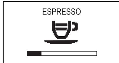
Product brewing stops automatically when the preset level is reached.
