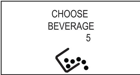
If the capsules are not removed from the drawer after several brewing cycles, the machine will stop. The display will show:
