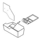
Clean the waste bin, the front panel and the overflow tray. Rinse under hot water and air dry completely.
