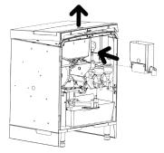
Reassemble the 3 soluble canisters. Lift the hood and slide the 3 soluble canisters at their position.
