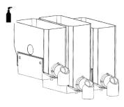
Clean the 3 soluble canisters. Rinse under hot water and air dry completely.
