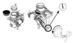
Reinstall the filter and the funnel on the brew group. Use the brewer tool to turn the dog drive counterclockwise to 11 o'clock.
