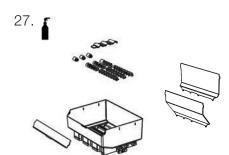
Disassemble the bean hopper prior to clean it. Rinse under hot water and air dry completely.
