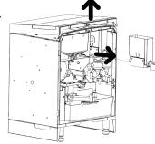
Gently lift the hood, pull the 3 soluble canisters out of the brewer. Empty each canister and take all parts apart.
