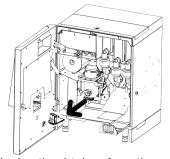
Unplug the 4 tubes from the spout. Unplug the spout from the brew group spillway. Remove the brown tube from the brew group funnel.
