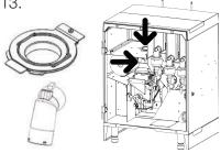
Unscrew and remove the rubber funnel bracket. Pull the coffee chute out from its socket.
