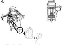
Use the brewer tool to turn the dog drive counterclockwise so the piston is at its lowest position.
