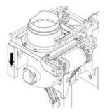
Push the locking pin down to release the brew group and on the right to keep the brew group unlocked.
