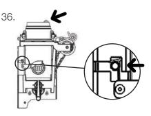
Reinstall the brew group and make sure the pin is on lock position. Reinstall the brown tube on the brew group funnel spring.
