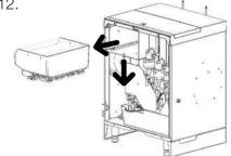
Pull down the bean hopper retaining pin. At the same time, pull the bean hopper outward.
