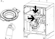
Install the rubber funnel and plug the coffee chute on its socket.
