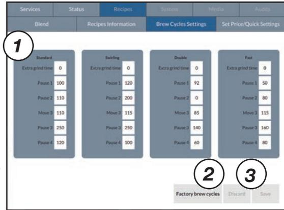
The Encore Venti has 4 different brew cycles. The brew cycle is automatically selected in accordance with the coffee and water quantities in the coffee-based recipe.
