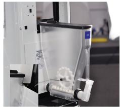
4.2 Disconnect blue tubes from mixing bowls. Then, for each mixing bowl, turn green ring counterclockwise about 1/8 turn.
