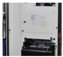
4.7 Return grounds tray container to machine. Reattach drip tray assembly to bottom and close door.
