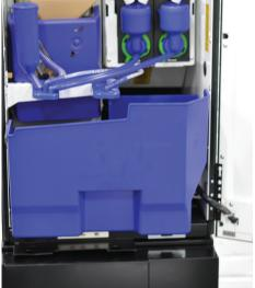
2.9 Reattach drip assembly to bottom of machine.
