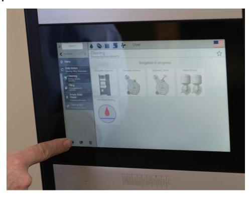
3.2 To reset waste bucket. touch question, "Have you emptied the waste bucket?" and allow machine to complete cycle. Touch icon in lower left corner to display Fast Action screen from Step 3.1. Next, touch question, "Do you want to rinse the machine?" and touch appropriate buttons to wash mixers and other functions as needed. Then, touch icon in lower left corner and touch "Confirm Exit from **Technical Menu**" on Fast Actions screen.
