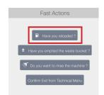
Press the "Have you reloaded?" button and adjust the level(s) of product(s) accordingly, then press the "Save" button to exit the menu.
