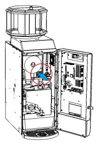
Air dry completely, then reinstall the elbow on its soluble ingredients canister. Close the door.
