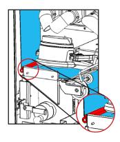
Install the new roll. Feed the paper under the left guide bracket of the brew group, under the brew chamber and under the wheel guides by gently lifting them using the yoke. Then close the door.
