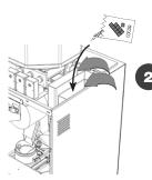
Remove the plastic hood. Fill up the soluble ingredients canisters **one at a time**. Reinstall the hood.
