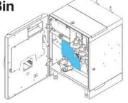
Cut the filter paper 6 inches below the yoke assembly with scissors.
