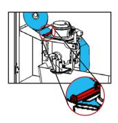
Install the new roll. Feed the paper under the left guide bracket of the brew group, under the brew chamber and under the wheel guides by gently lifting them using the yoke. Then close the door.
