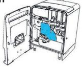
2 Cut the filter paper 6 inches below the yoke assembly with scissors.
