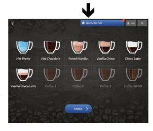
\*When using the internal waste bin provided with the unit, Cafection recommends setting the counter to 25 cycles using standard 8, 10 and 12 oz cups.
