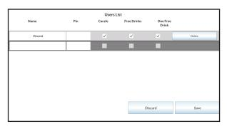
If at least 1 user is created, a user icon appears on the selection screen (top right corner). When the user presses on this button, a pop-up window with a numeric keyboard appears. Once the user has entered a correct PIN, he will be able to activate the authorization(s) he has been granted. If the user enters an incorrect PIN five times in a row, the user icon will be locked. To unlock it, enter and
