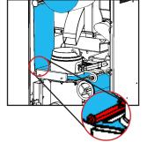
Install the new roll. Feed the paper under the left guide bracket of the brew group, under the brew chamber and under the wheel guides by gently lifting them using the yoke. Then close the door.
