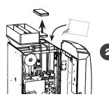
Open the door and remove the plastic hood. Remove lids of the soluble ingredients canisters **one at a time** and fill them up.
