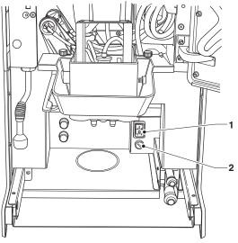
Fig. 43 1. Main switch 2. Line fuse
