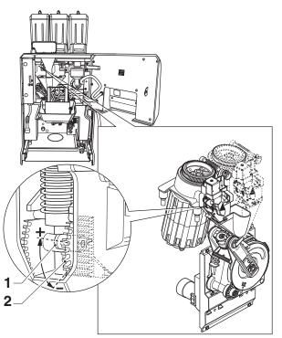
Fig. 27 1. Dose adjustment lever 2. Dose adjustment
