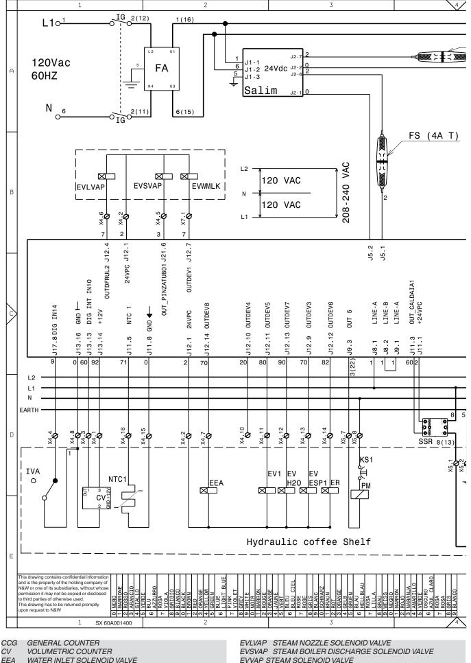
CV FFA WATER INLET SOLENOID VALVE EEAVAP WATER INLET SOLENOID VALVE FOR STEAM ER COFFEE DISPENSING SOLENOID VALVE ESP1-. DRAIN SOLENOID VALVE EV1-.. INSTANT SOLENOID VALVES EVAIR AIR SOLENOID VALVE EVH2O WATER SOLENOID VALVE
