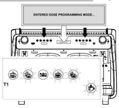
To carry out a new programming of the other coffee doses T2-T4-T5-T6 (if the programming time-out of 30 seconds has not been exceeded), it is sufficient to repeat the same sequence of operations carried out for the T1 key.
