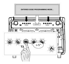
Press the key corresponding to the dose to be programmed (key TI for example) within 30 seconds (programming time-out). The LED light of the dose being set keeps switched on together with the T3 key of the keypad of the group to be set. During this stage and for the entire coffee dose programming time duration, the solenoid valve and the pump are activated.
