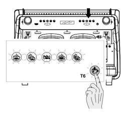
It is possible to stop the brewing before the programmed product quantity is reached by pressing again the dose button used for dispensing the product.
