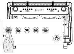
The brewing in progress can be suspended before actually reaching the desired programmed product quantity by pressing any of the dose keys on the keypad of the group used for product brewing.
