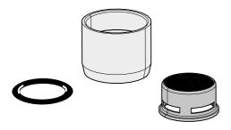
Screw the airing filter of the hot water dispensing spout (11).
