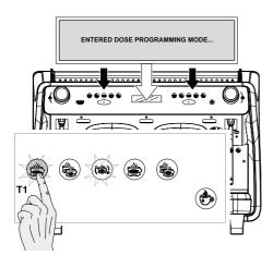
After pressing the TI key, the brewing starts. After reaching the desired coffee dose, press the TI key again to stop brewing the coffee dose. This way the new value is saved by the pulses of the dose. Both the solenoid valve and the pump are deactivated thereby suspending product brewing. The LED relating to the programmed key turns off.
