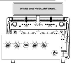
Press the T3 key again to immediately exit the programming stage.
