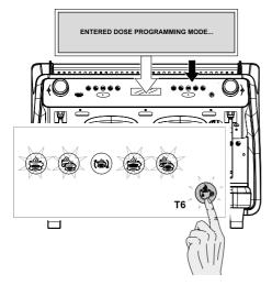
After pressing the T6 key, water dispensing starts. When the desired tea dose has been reached, press the T6 key again to stop dispensing the water dose. This way the new value is saved by the pulses of the dose. Both the solenoid valve and the pump are deactivated thereby suspending product brewing. The LED relating to the programmed key turns off.
