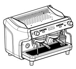
By pressing the T6 key, the corresponding dispensing solenoid valves are activated until the previously programmed product quantity (time control) is reached. The LED corresponding to the button of the selected TEA dose will be steady on during the whole hot water dispensing stage.
