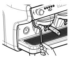
Clean every hole of the nozzle by means of a bottlebrush to remove any residuals.
