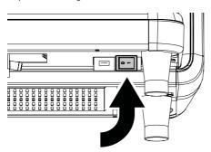
If set to the "I" position the machine turns on (electrical functions enabled). If set to the "O" position the machine turns off (electrical functions disabled).
