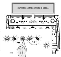
Press T6 key within 30 seconds (programming time-out). The LED of button T6 is on and flashing. During this stage and for the entire tea dose programming time duration, the solenoid valve and the pump are activated.
