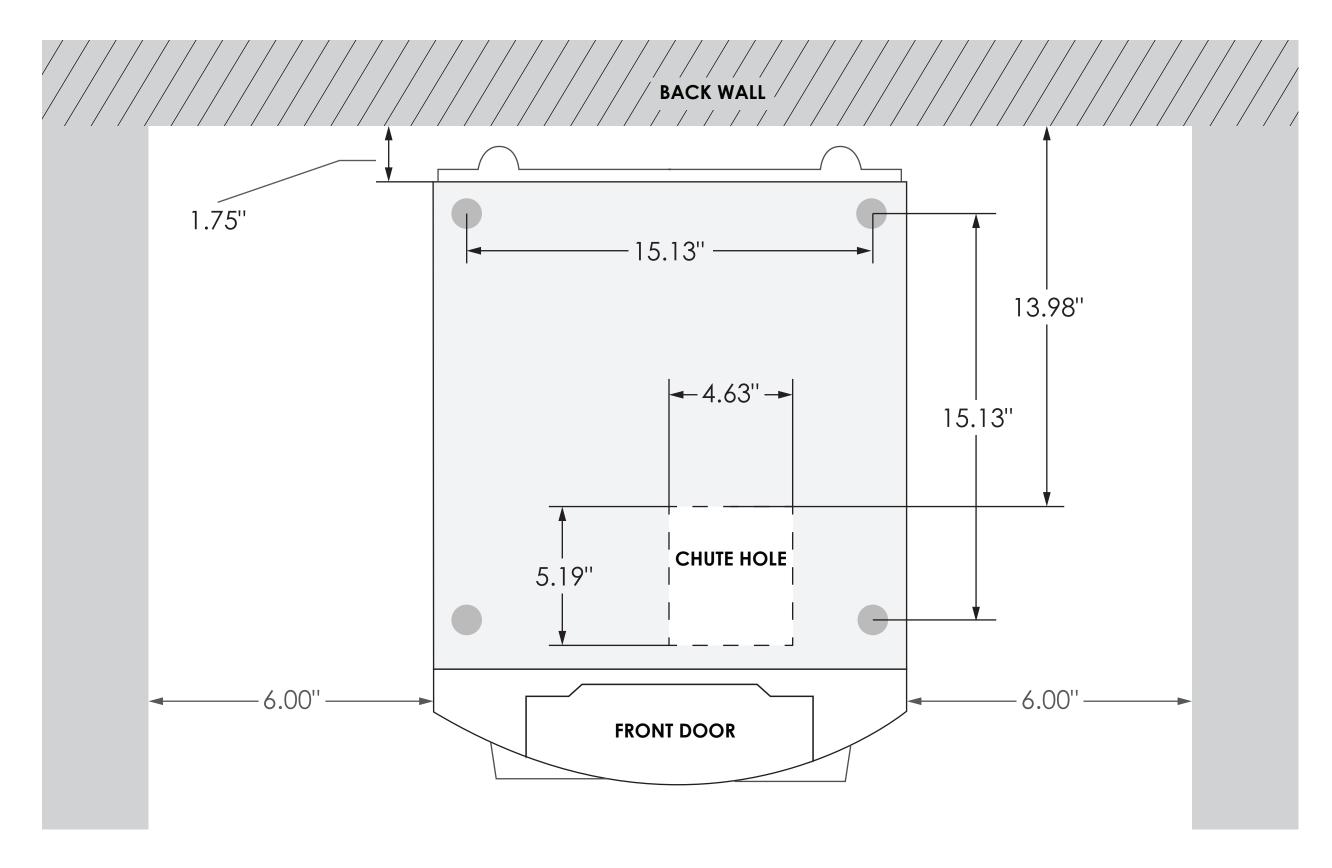
"HOLE EDGES SHOULD BE SEALED WITH SILICONE OR AN APPROPRIATE SEALANT FOR PROTECTION AGAINST WATER DAMAGE"
