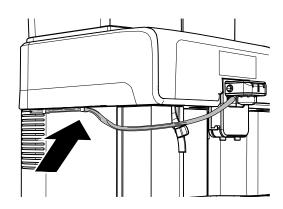
If the coiner is installed, fix the tube as shown in the figure by using the previously removed cover.
