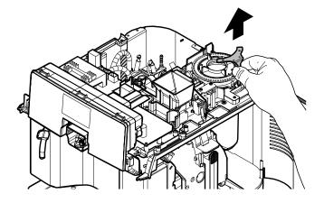
Using long nose pliers, remove the coffee grinder from its support grommets.  $\,$
