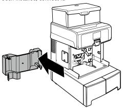
Insert the front cover and fix it by means of the screw previously removed. Insert the coffee dispensing spout. Reassemble the drip tray.
