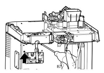
Removing the sol. valves assembly.
