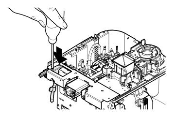
Remove the hot water/steam pipe assembly.
