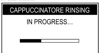
The machine performs a Cappuccinatore rinse cycle. The bar shows the rinsing progress.
