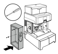
The connecting cable must be properly inserted in the box.
