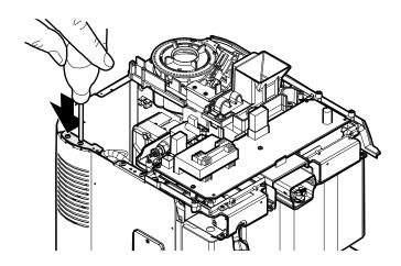
Remove the coffee boiler assembly and disconnect the wires and pipes.
