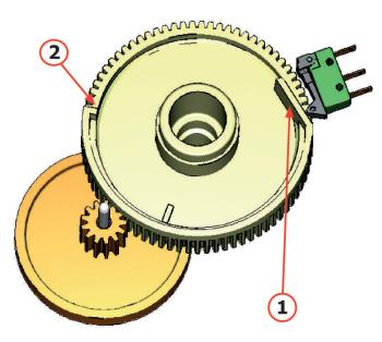
The gearmotor is driven by a DC motor acting on the smallest double gearwheel wheel through a worm screw.
