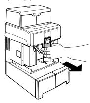
Remove the front cover by pushing on its sides to disengage the fixing elements.
