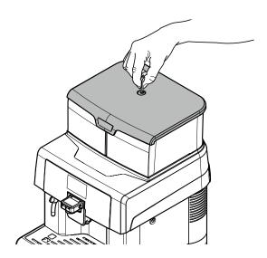
After unlocking the lid, lift and remove it.
