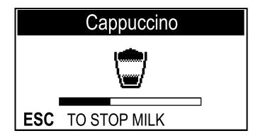
The machine dispenses frothed milk. Dispensing can be stopped by pressing the "Cappuccino" button or the "ESC" button.
