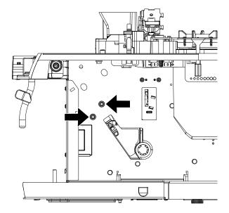
Remove the boiler pin.
