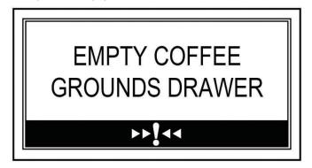
In this case, the machine does not allow beverages to be dispensed. In order to dispense beverages, the coffee grounds drawer must be emptied of used coffee.
