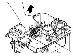
Disconnect the water inlet pipe.
