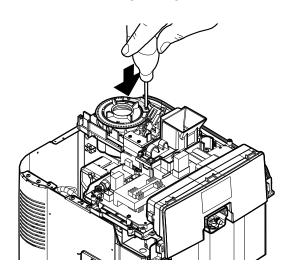
Remove the grommet from the grinder adjuster lever.
