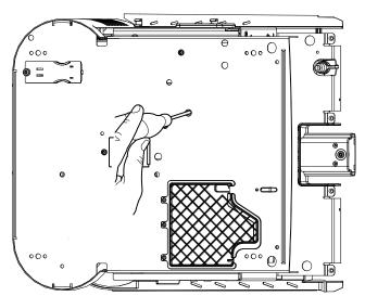
Remove the discharge solenoid valve.
