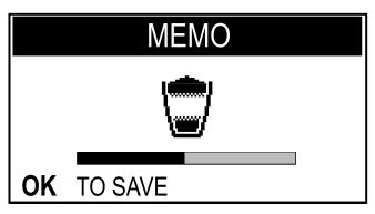
Press the "OK" button when the desired amount of coffee is reached in the cup. Now the "Cappuccino" button is programmed. Each time it is pressed, the machine will brew the same amount that was just programmed.
