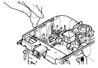
Remove the pipe locking plate.
