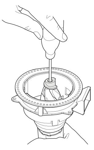
Remove the increment screw and its fasteners.
