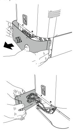
Disconnect the pipes and wires from the inlet solenoid valve.
