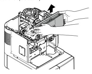
Remove the front panel assembly upper cover.
