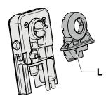
Insert the tube on the left-hand side of the fitting.
