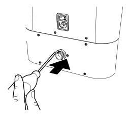
Remove the inlet solenoid valve.
