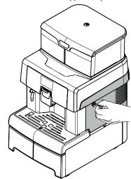
Remove the brew group by pulling it by the handle and pressing the «PRESS» button.
