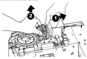
Disconnect the microswitch wiring and remove it from its housing.
