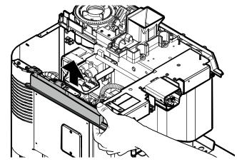
Remove the coffee boiler as explained in "Disassembling the coffee boiler" section.
