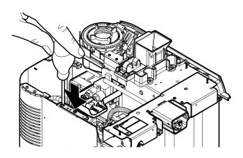
Remove the hot water/steam boiler assembly and disconnect the pipes and wires.
