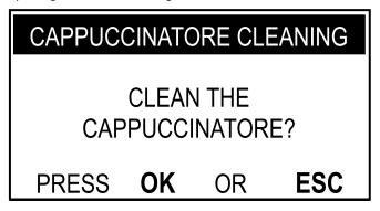
Press the OK button to start the cleaning cycle of the Cappuccinatore and place a container under the coffee dispensing spout. Follow the instructions on the display.
