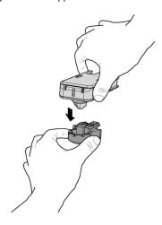
Turn and lift the Cappuccinatore cover and remove it from the Cappuccinatore body.
