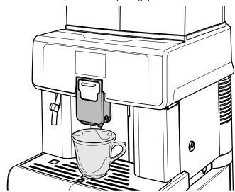
Confirm by pressing the "OK" button to start the preparation. After brewing, remove the cup of coffee.
