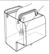
Put the filter into the empty tank. Press it to its limit stop.
