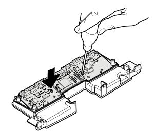
Disconnect the wiring.
