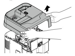
Disconnect the 2 silicon pipes and the water level sensor wiring harn. Remove the screw shown in figure using a Torx T10 screwdriver.
