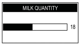
Press the "DOWN" button or the "UP" button to move the bar and select the desired value; the number on the side identifies the bar value (in seconds). Then press the "OK" button to confirm and exit. Press the "DOWN" button to select the "PAUSE" menu.
