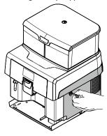
Remove the brew group by pulling it by the handle and pressing the «PRESS» button.
