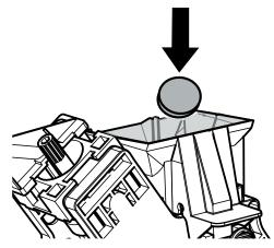
After placing the tablet in the brew group, press the "OK" button to confirm.
