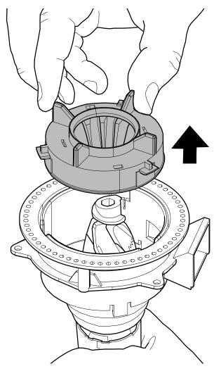
Remove the upper grinder from its supports with a flat-head screwdriver.
