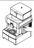
The reference marks indicate the amount of ground coffee which has been set. You can set different amounts with the following references:
