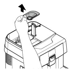
Remove the coffee bean hopper lid sensor (if available) using a flat-head screwdriver.
