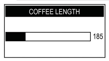
Press the "DOWN" button or the "UP" button to move the bar and select the desired value; the number on the side identifies the bar value (in pulses). Then press the "OK" button to confirm and exit. Press the "DOWN" button to select the "MILK QUANTITY" menu.
