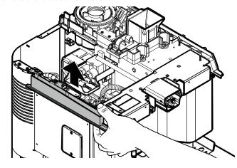
Remove the 2 screws shown in figure using a Torx T10 screwdriver.
