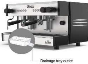
Remove the drainage tray and connect the corrugated hose, supplied with the machine, to the drainage tray outlet (see figure), before finally connecting the other end to the general drainage system of the establishment.
