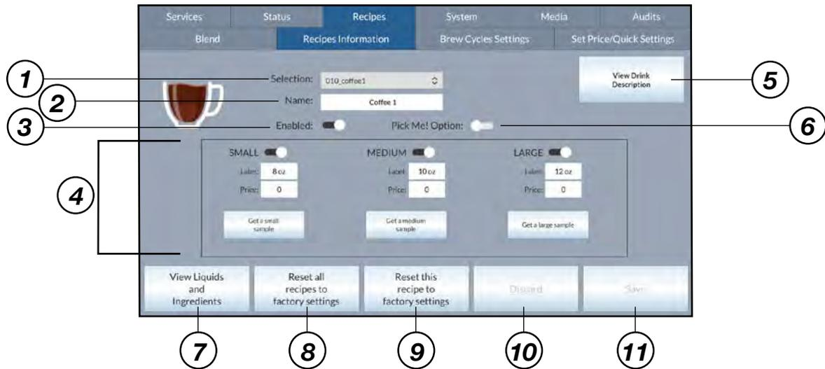
1. This drop-down menu is used to choose the recipe requiring modifications. Coffee 1, 2 and 3 refer to bean hopper sections 1, 2 and 3 (from left to right).
