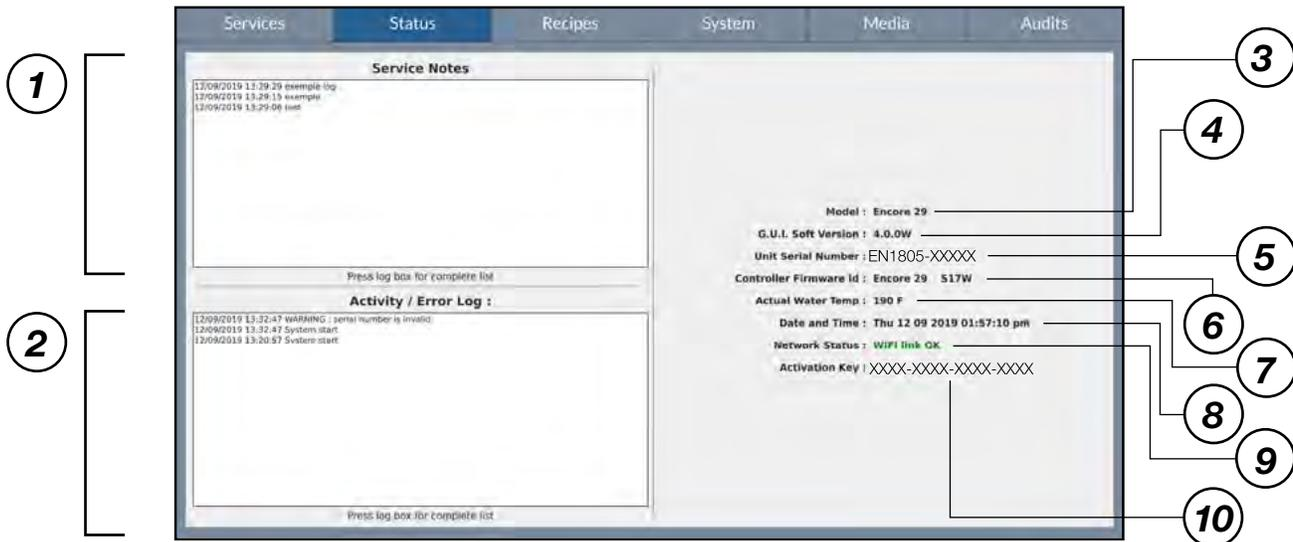
1. Service Notes. Allows the technician to enter the servicing that has been performed on the machine. An alphanumeric keyboard will appear when pressing the text box.
