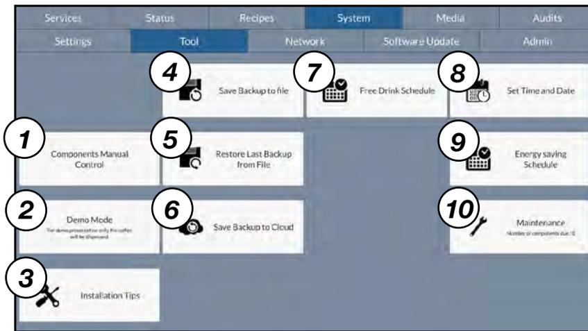
1. This button is used to enter Manual Control mode and manually test the machine's components.
