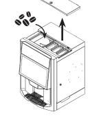
Remove the lids of the soluble ingredients canisters one at a time and fill them up.
