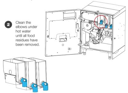
Air dry completely, then reinstall the elbows on their proper soluble ingredients canisters.
