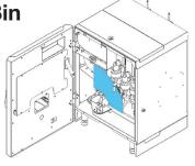
Cut the filter paper 6 inches below the yoke assembly with scissors.
