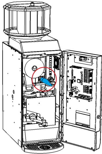
**3** Air dry completely, then reinstall the elbow on its soluble ingredients canister. Close the door.
